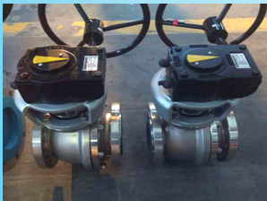
Wanhua Chemical Group Co.,Ltd. (Ningbo) MDI Viscous Material Shut-off Valve Sept.2013
